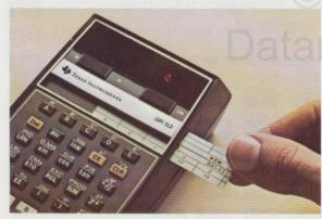
3. Slide the magnetic card into the window. A-side above keys **A** through **E** .
