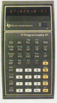
Trigonometric functions. Statistical functions. Nine levels of parentheses and the ability to store up to four pending operations let you handle even complex equations quickly and easily.
