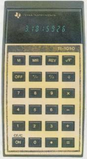
having to shift decimal points — perfect for figuring discounts and add-ons. And there's a time-saving automatic constant that lets you do repetitive calculations without having to reenter numbers. And the full-function memory and algebraic entry system makes calculating investment decisions a simpler task.
