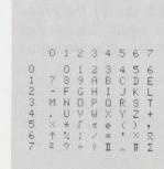
The PC-100A with the TI Programmable 58 or 59, provides print capability for 64 characters (including blank space). Each character is entered by means of a 2-digit address code. Maximum line length is 20 characters.
