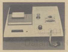
In the Manual Selector, modules are housed in numbered locations at the bottom of the selector. Once the modules are in place, it is an easy matter to dial the desired module per the rotary switch at the top of the selector. Although the Manual Selector will operate on a stand-alone basis, it has been designed to fit into the well of the PC-100A/C printer with the battery removed.
