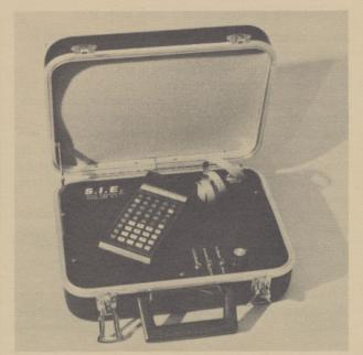
Two operating modes allow for 'on demand' speech or constant speech output and can be used to prompt the user during program execution. Any existing TI-58C/59 may be easily attached to the SIE Speech Adapter by removing the original battery pack and replacing it with a special adapter battery pack. The Speech Adapter itself is contained in a 12" X 8" X 3" attache case with space provided for the calculator and power cord.
