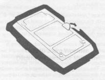
The exposed metal contacts on the battery pack are the battery terminals. Care should always be taken to prevent any metal object from coming into contact with the terminals and shorting the batteries.
