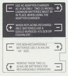
Rechargeable Battery Operation — The TI-2500-II is supplied with two fast charge nickel-cadmium batteries installed in the upper section of the battery compartment. These batteries should be left in the calculator at all times unless it becomes necessary to replace them. The batteries may be recharged using an AC 9130 Adapter/Charger. The rechargeable batteries cannot be recharged if alkaline batteries are installed in the lower section of the battery compartment.
