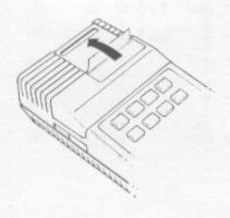
Lift the old roll of paper from the calculator and cut or tear the paper to separate the end of the roll from the paper remaining in the printing mechanism.
