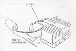
Place the new roll of paper in the paper compartment so that the paper unrolls from the bottom of the roll.
