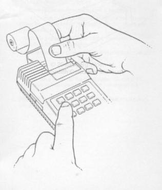
Place the new roll of paper back into the paper cradle and close the paper access door to complete paper installation.
