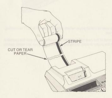
2. Place the new roll of paper behind the calculator so that the paper unrolls from the bottom of the spindle. If there is paper remaining in the printer, use this step to install paper and skip step 3. Otherwise, proceed with step 3.
