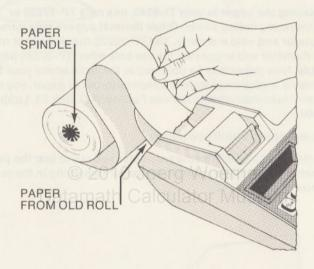
3. Use this step to install paper when a piece of paper is NOT remaining in the printer.
