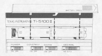
Realign the hooks on the cover with the grooves along the battery compartment. Replace the cover by sliding it to the left.
