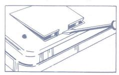
Remove the battery compartment door by prying gently with a small screwdriver, key, coin, or similar object. Follow the instructions on the floor of the battery compartiment.
